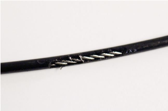
A TEAR IN THE CABLE COVER
