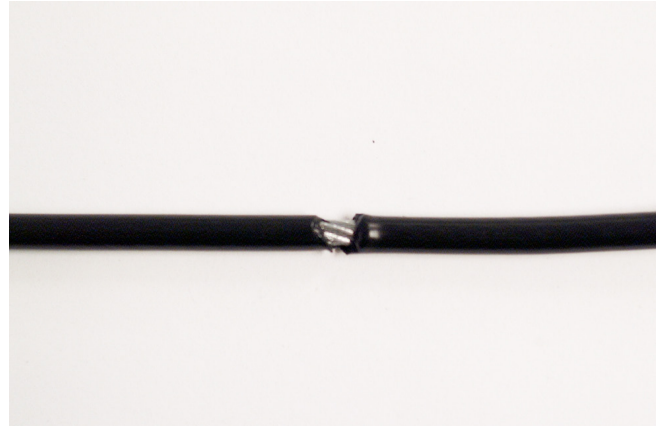
A CRACK IN THE CABLE COVER
