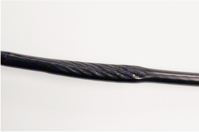
"NECKING", STRECHED CABLE COVERING
