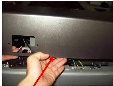
remove the motor cover
