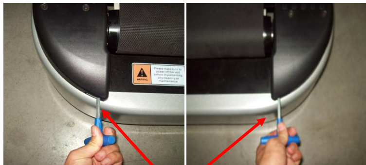
Use 6 # socket head wrench to adjust the running belt tightness counterclockwise, loosening the running belt
