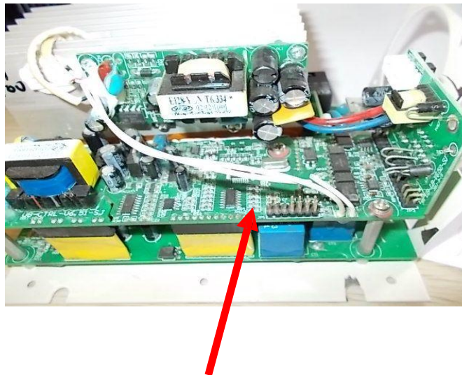
Control panel for incline
