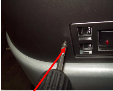
Remove the cross pan head screw
