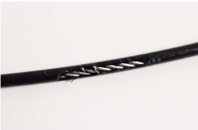
A TEAR IN THE CABLE COVER
