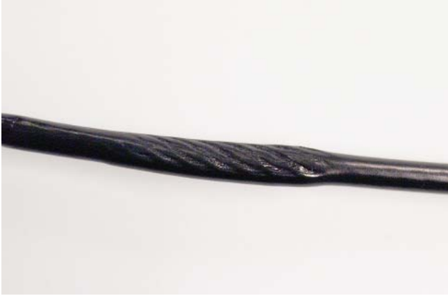
"NECKING", STRETCHED CABLE COVERING
