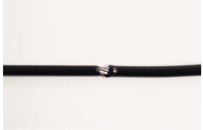
A CRACK IN THE CABLE COVER
