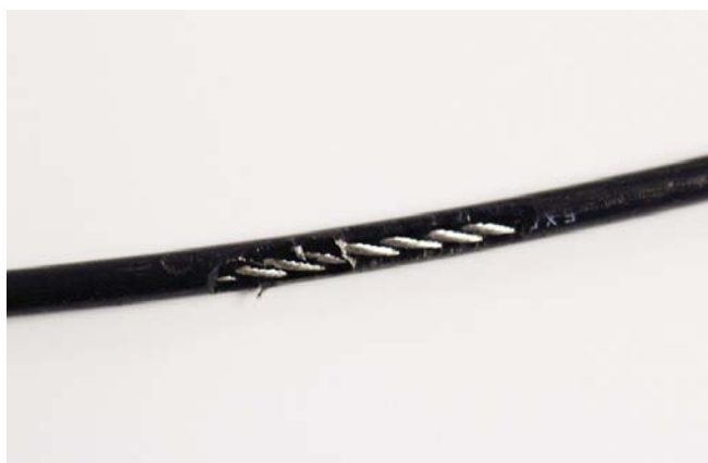
A TEAR IN THE CABLE COVER
