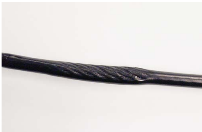
"NECKING", STRECHED CABLE COVERING
