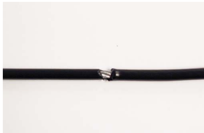
A CRACK IN THE CABLE COVER
